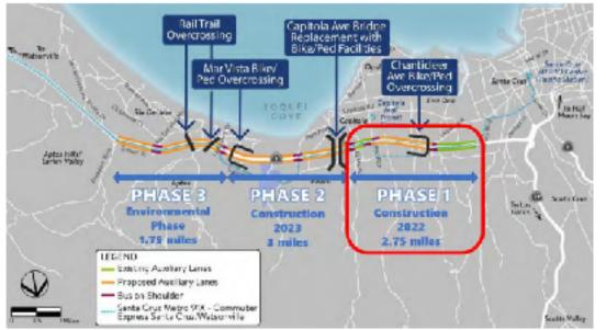
Figure 1 - Phase 1 Project includes auxiliary lanes and a bus on shoulder facility in both directions of Highway 1 (41" Avenue to Soquel Drive), retaining walls, soundwalls, and a new bicycle/pedestrian overcrossing at Chanticleer Avenue
